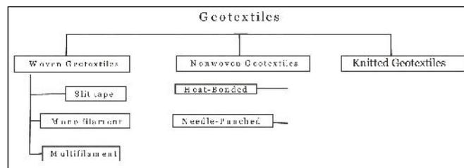
Geo textiles are generally made up of woven, non-woven and knitted type of fabrics.
